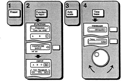
4 Adjust the time/div and Delay values as needed.
