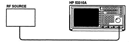
1 Set the RF source to output a power level 30 dB below the nominal power level of the transmitter (as determined in the previous section) and at the same frequency as the transmitter.
