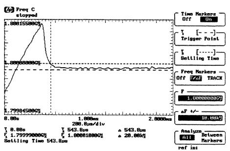
Hint: Once a single measurement has been acquired and the HP 53310A is stopped, you can change the  $\Delta F$  value and see the settling time for different tolerance band values.
