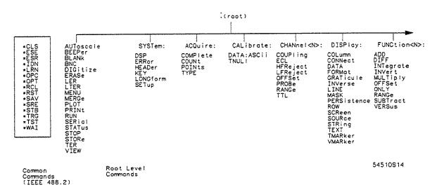
This instrument contains two identical channel subsystems and two identical function subsystems. The "N" in the Channel header must be 1 or 2 and the Function header must be 1 or 2.
