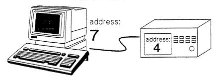
DEVICE ADDRESS = (Interface \* 100) + Instrument = (7 \* 100) + 4 = 704
