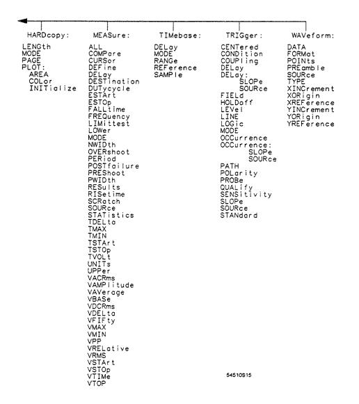
The common commands are commands which are independent of the tree and do not affect the position of the parser within the tree. Root level commands are commands that reside at the root of the command tree. They are prefaced by a colon that puts the parser at the root level. Finally, the subsystem commands are commands that are grouped together under a common node of the tree, such as the TIMEBASE commands.
