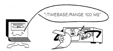
Messages for programming the oscilloscope appear as ASCII character strings embedded inside I/O program statements. Each message consists of a device address, a program message, and a terminator. The address uniquely identifies one of the instruments on the bus while the program message specifies the action to be taken by that instrument.
