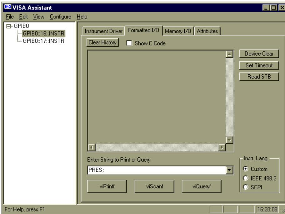
2. To further verify GPIB operation, send a preset command to the analyzer by doing the following in the VISA Assistant window:
