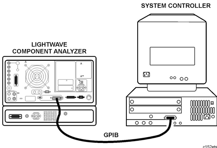
2. Switch on the computer, and launch HP BASIC or HP BASIC for Windows.
