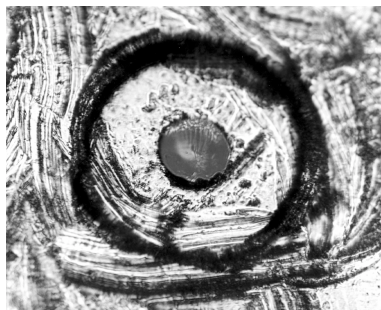
Figure 1-6. Damage from improper cleaning.
