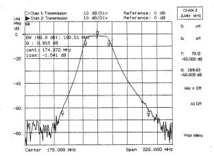
The figure to the left contains the result of the filter bandwidth measurements just performed. The filter's shape factor can be calculated by dividing the filter's 60 dB bandwidth (channel 2) by the filter's 3 dB bandwidth (channel 1). In this example (190.5 MHz)/(51.7 MHz) = 3.68:1.
