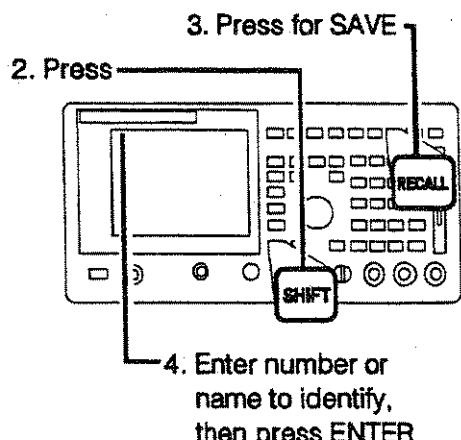
NOTE: The number of changes made to the screen determines memory consumption.
