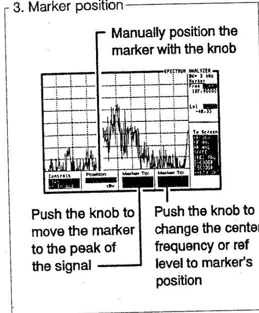
Push the knob to move the marker to the peak of the signal
