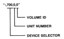
The device selector refers to the address of your disc drive. The first number is 7 as long as you are using the internal HP-IB connection. The last two numbers are the address of your disc drive. These numbers may vary from 00 to 07, depending on the address setting. In this example, the disc drive address is 00.
