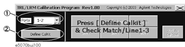
Figure A-3 TRL/LRM main control panel
