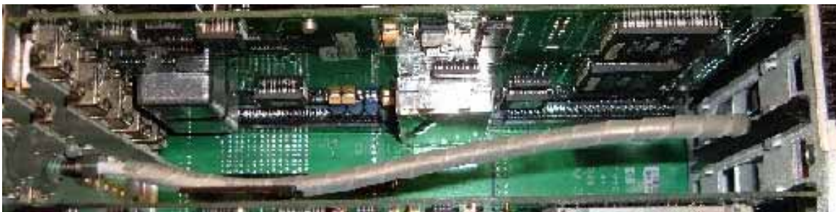
Figure 7 Spiral Wrapped Cable to Option H3B Rear Panel
