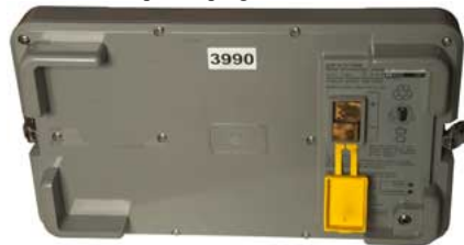
Fig 15 The device behind the yellow cover is a flat spring contact that will press up against the adapter. The center pin of the recessed charge plug is too big to accept a 5.5 x 25 DC power plug. What connector is it?
