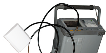
Fig 22 SA and Wi-Fi boxes the same locations as Fig 21. Just changed from whip to Wi-Fi Panel antenna.
