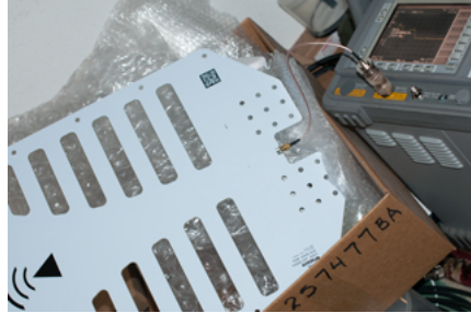
Fig 26 RF Space TSA400 UWB ant -29.24 dBm
