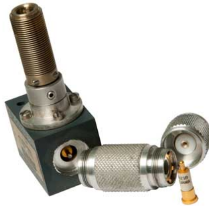
Fig 2 1N21B mixer diode shown. The diode inside the block is 1N416B harmonic generator
