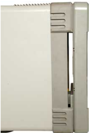
Fig 17 There is a gap so cables, like RG-58 can be used on the rear connectors.
