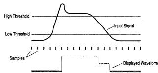
• A tolerance band exists below the high threshold and above the low threshold. An input signal value within a tolerance band can be displayed as either a logic level or a tristate level. For example, if an input signal level is in the high tolerance band, the logic level in the waveform can be either a high level or a tristate level. The width of the tolerance band depends upon the logic family used and is defined in the specifications on page 35.
