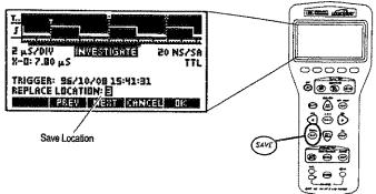
• There are 10 waveform storage locations, numbered from 1 to 10. Press TEXT or TAXIII to select a storage location.
