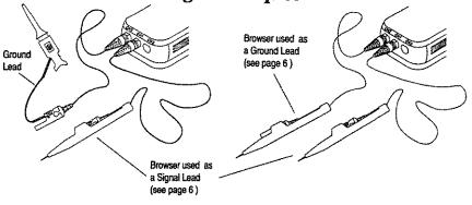
You can use the ground connection from either Channel 2 or Channel 3 for low frequency Channel 1 operations. All ground connections are common (not isolated) to all channels.
