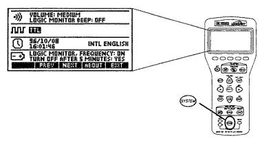
To use System Setup, move the highlight (white text on a black background) to the area of interest and then change the values for that setting. The Logic Family setting, TTL, is highlighted in the screen above.
