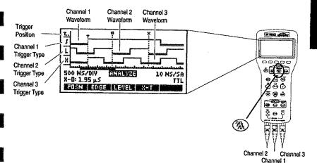
• In Analyze, you have more control over waveform triggering. You can set the trigger conditions for all three channels. Press FOFF or FOFF to choose the trigger types, then select the channel for the trigger type using one of the FOFF menu keys. The trigger position and trigger types are described on page 12.
