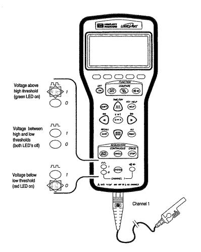
Use the logic monitor with the browser to quickly locate active or stuck nodes, power supplies, and grounds. Page 5 shows how to use the probes.
