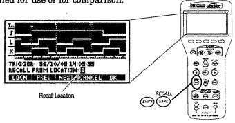
There are 10 waveform storage locations, numbered from 1 to 10. Press NEW or FREW to select a storage location. When the desired location is selected, press to recall the waveform and setup.
