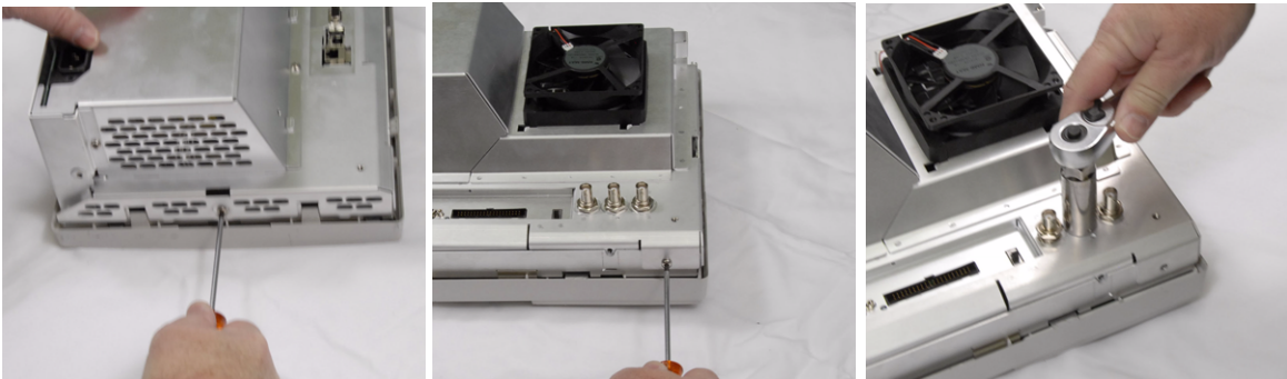
Figure 19 Removing the rear deck assembly
