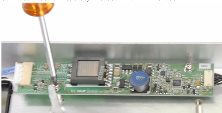
Figure 24 Removal of inverter board
