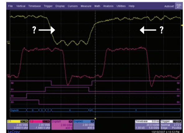
LeCroy WaveSurfer's slow update rate misses the signal jitter and metastable state.
