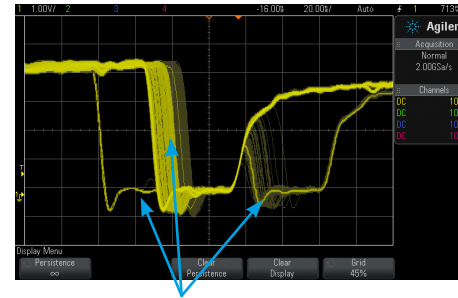
Infrequent glitch and signal jitter captured after 2 seconds on 2000 X-Series with > 50,000 wfms/s
