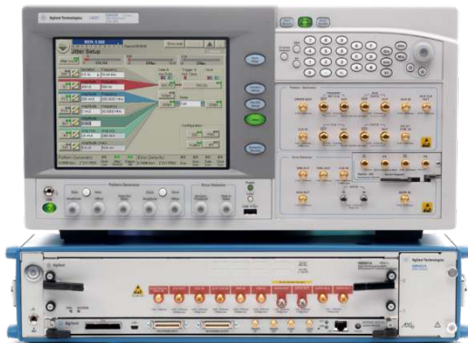
The M8061A multiplexer can be used to extend the data rate of J-BERT N4903B to 28.4 Gb/s.
