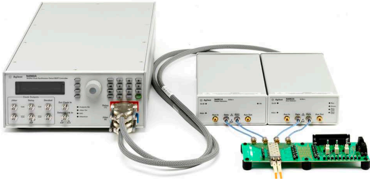
Figure 1. For 16x Fibre Channel (16 GFC) for transceiver testing.
