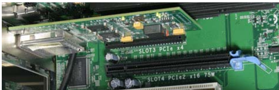
Figure 63 An example PC’s x8 (x4 mode) and x16 (x16 mode) PCIe slots
