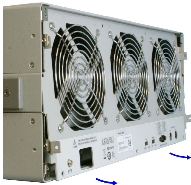
Figure 79 The base of the rear panel is slid out first
