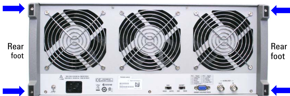
Figure 77 Removal of the two rear feet
