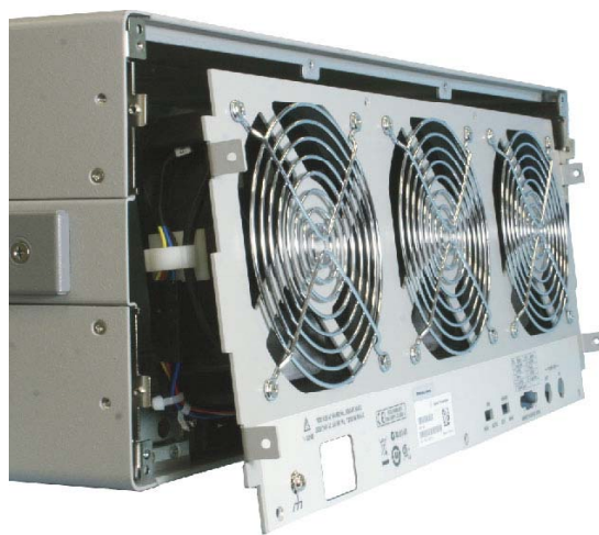
Figure 80 Removal of the rear panel
