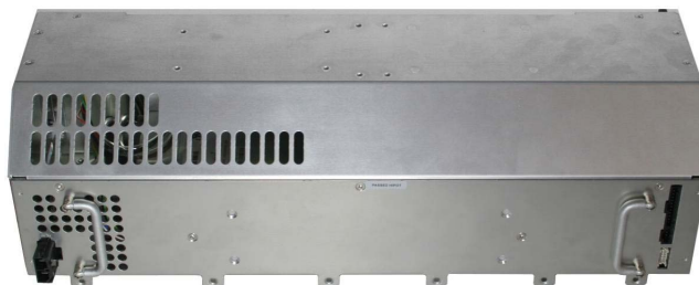
Figure 75 Chassis power supply
