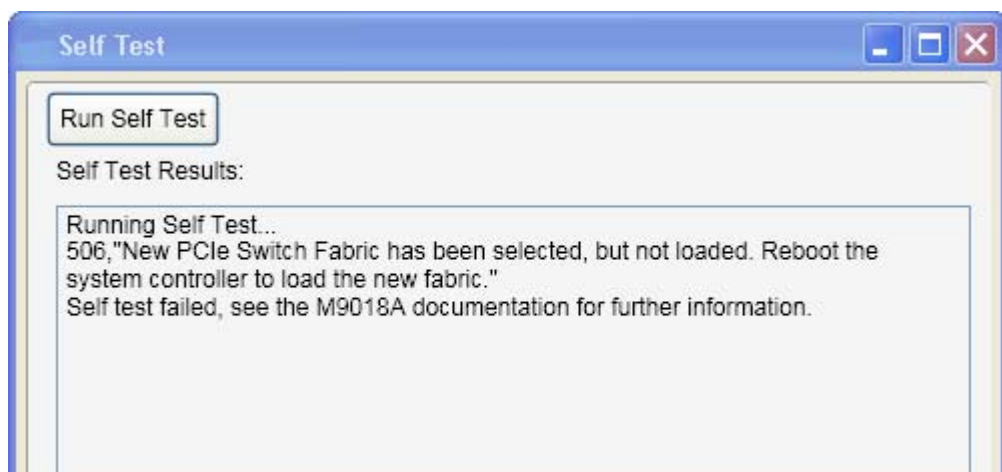
Figure 46 If self test is run prior to rebooting your computer, it will detect that the computer needs to be rebooted
