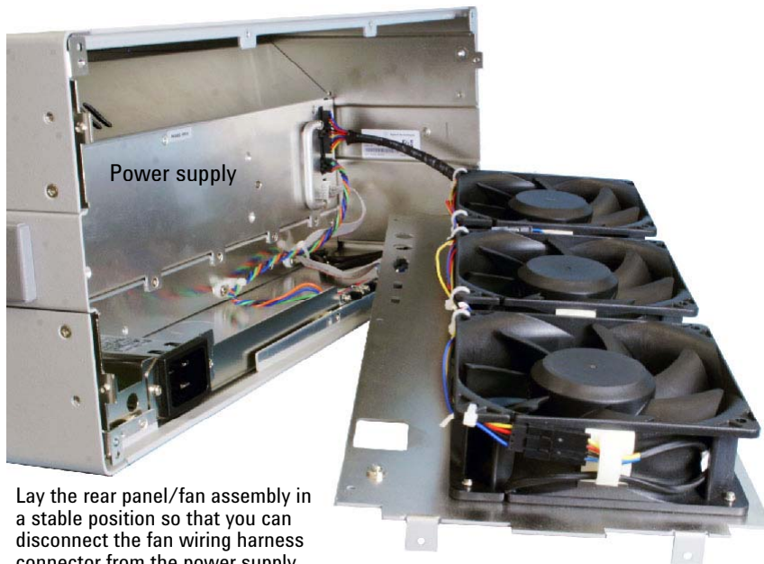
Figure 81 Positioning of the rear panel/fan assembly in preparation for disconnecting the fan connector
