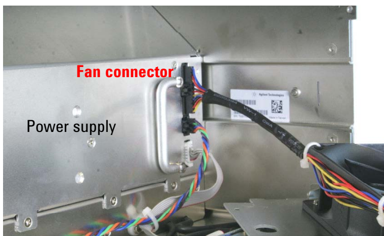
Figure 82 The fan connector is the top-most connector.
