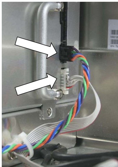
Figure 88 Remove the two remaining power supply connectors
