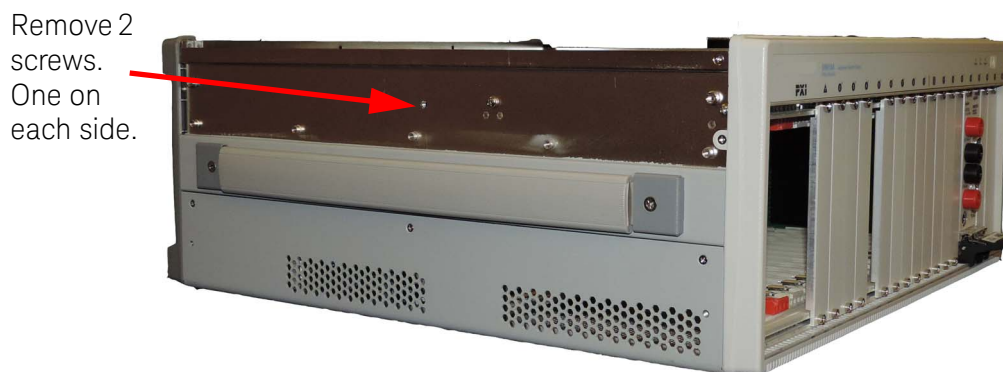
Figure 86 Remove two screws inside of chassis securing power supply
