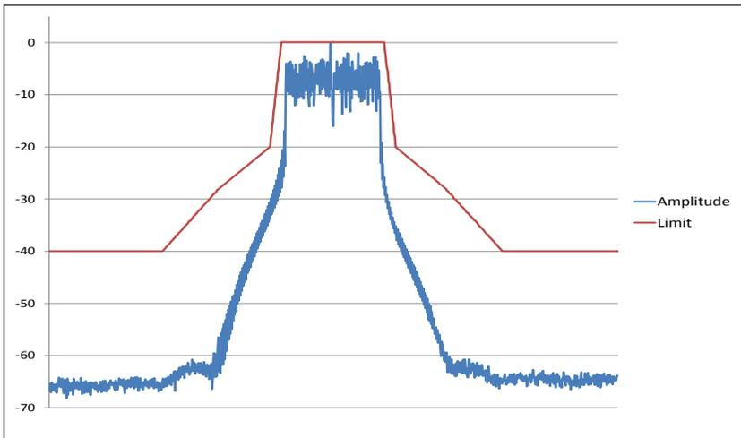
Figure 12. WLAN 802.11a/g SEM at 5.5 GHz, 20 MHz bandwidth.
