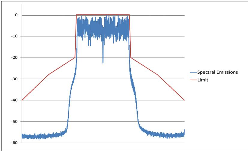
Figure 10. WLAN 802.11ac SEM at 5.8 GHz, 80 MHz bandwidth.
