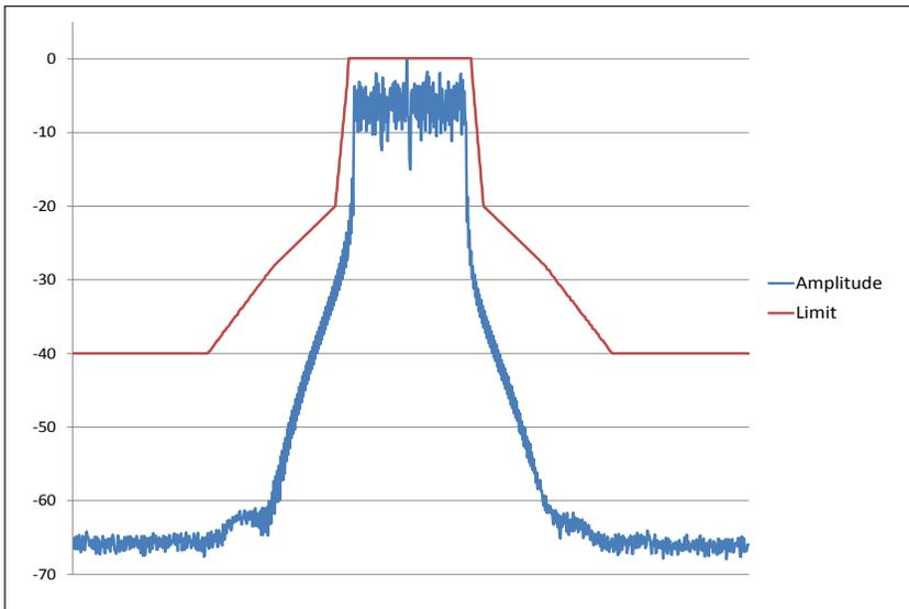
Figure 11. WLAN 802.11a/g SEM at 2.4 GHz, 20 MHz bandwidth.
