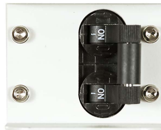
Circuit Breaker Closed (ON)
