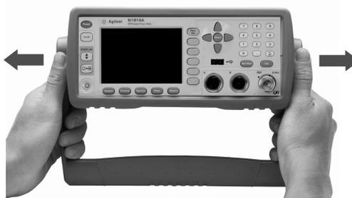
To remove the handle, refer to Rack Mounting the Power Meter on page 32.
