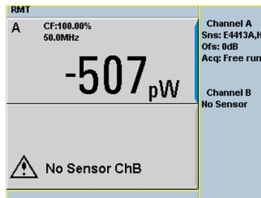
Diagram shows display with an E-Series E4413A power sensor connected.
