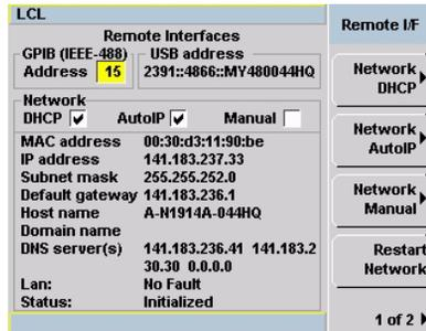
**Figure 1-5** Typical GPIB Remote Interface
