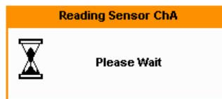
This message does not appear when connecting an 8480 Series power sensor.
