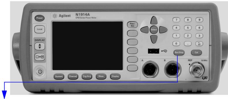
These keys and connectors are associated with the measurement channels and are located on the right-hand side of the front panel.
