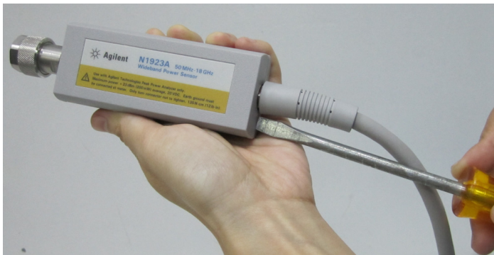
Figure 4-2 Removing the N1923/4A shell
