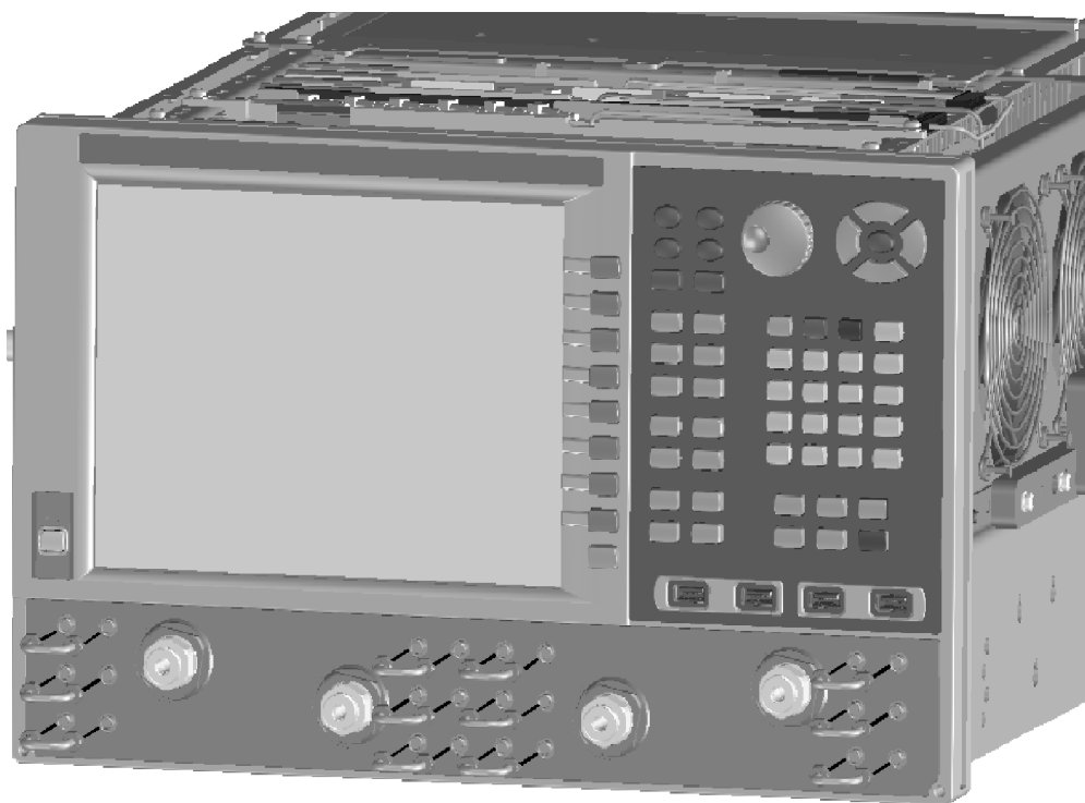
Figure 5 Front Panel Jumper Cables Installation
