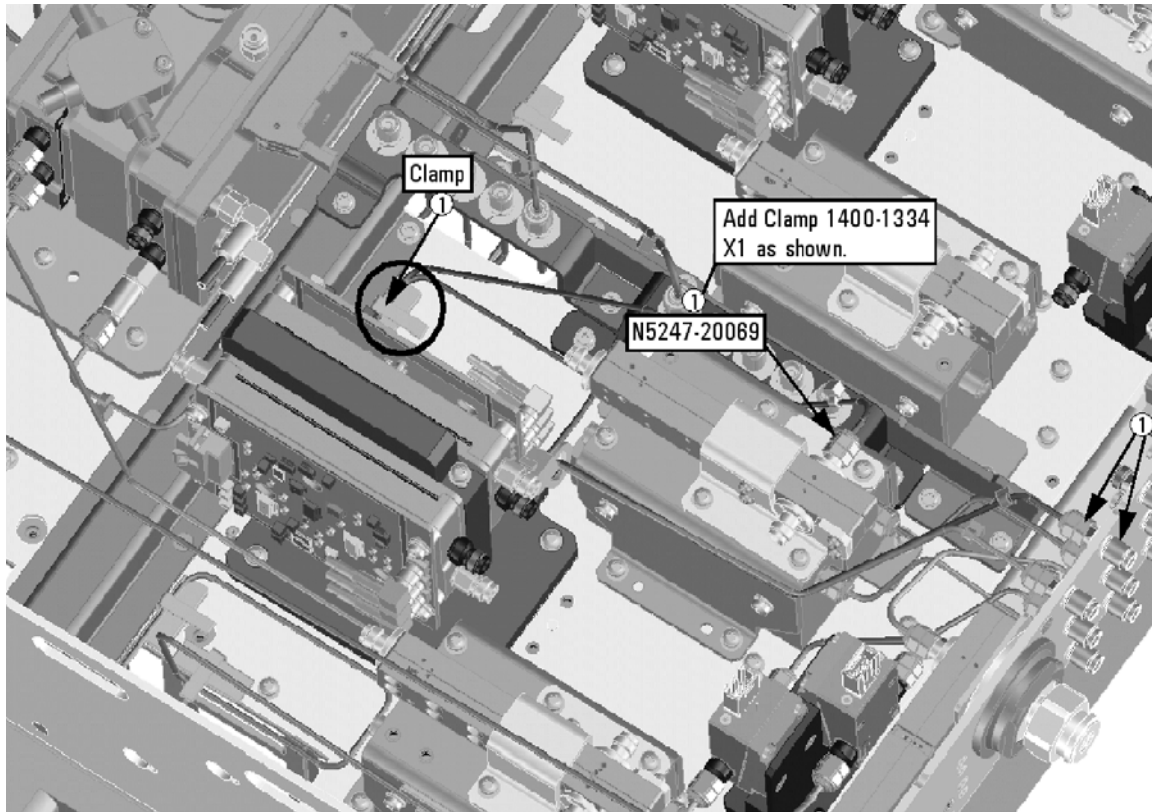
Figure 10 Location of Cable Clamp to Secure W41 (N5247-20069)
