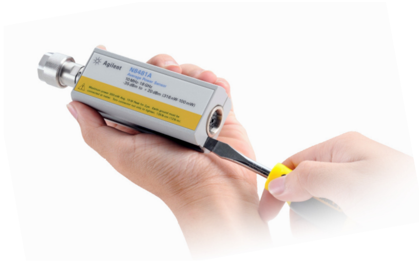
Figure 3-2 Removing power sensor shell
