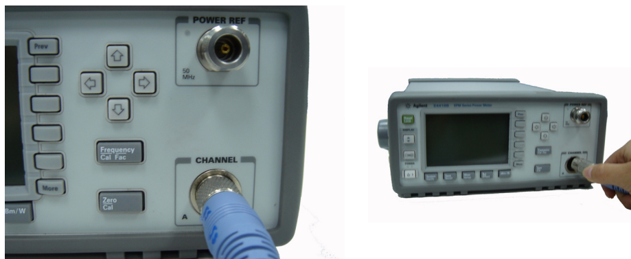
Figure 1-2 Connecting a sensor cable to power meter
