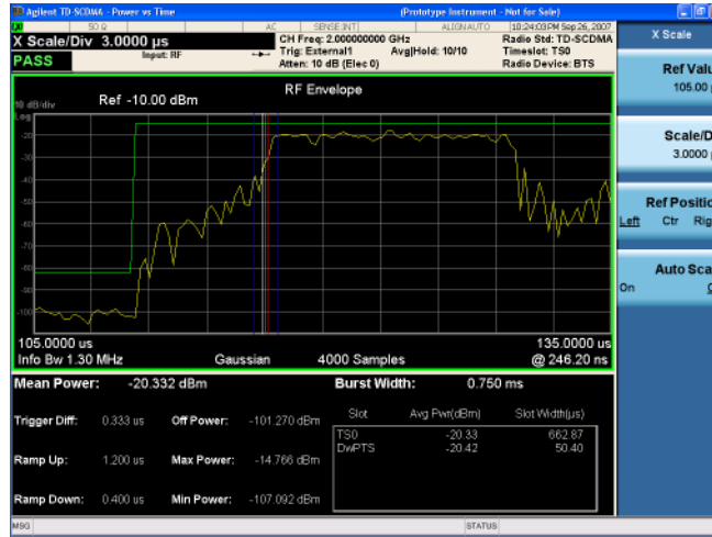
Power vs. Time - Zoom in (Ref Value = 105 \mu s, Scale/Div = 3 \mu s)
