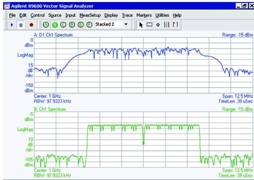
Figure 4-49 Frequency domain response of a OFDM signal without using an instrument trigger (upper trace) and using a trigger to set the beginning of the downlink frame (lower trace). (Example from the Keysight 89600).
