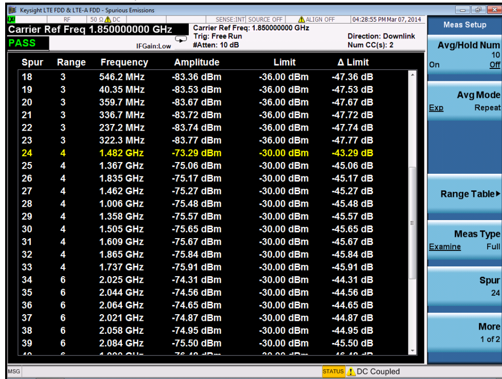
Figure 2-15 LTE FDD & LTE-A FDD Downlink Spurious Emissions Measurement - Numeric Result Screen
