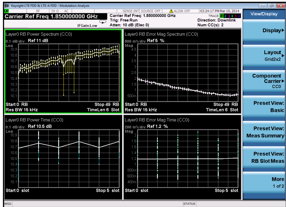
Figure 2-31 Modulation Analysis Measurement Result - RB Slot Meas Preset View
