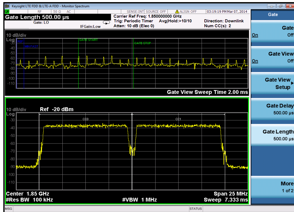
Figure 2-6 Monitor Spectrum Measurement - Gate View
