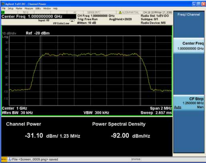
Figure 2-2 Channel Power Result – Bar Graph Off
