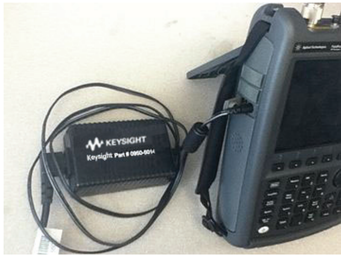
Figure 2. The FieldFox connected to its DC power supply
