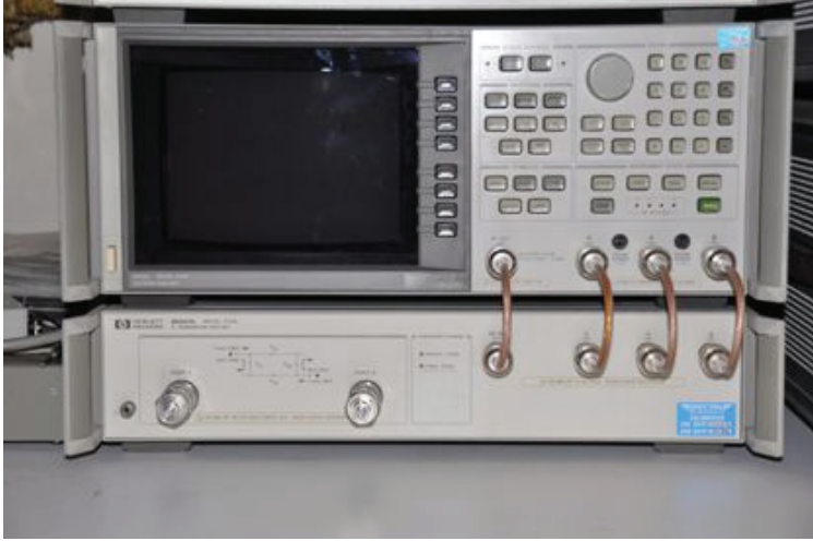
Figure 7. An HP-8753C 6 GHz network analyzer on top with its matching HP-85047A S-parameter test set below. The RF, R, A, and B signal connections between the two instruments are clearly visible.
