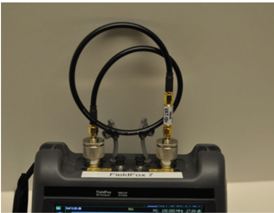
Figure 9. Measurement of a coaxial attenuator using the FieldFox
