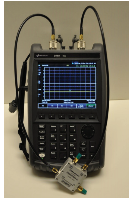
Figure 6. Measurement of the Mini-Circuits ZFBDC20-62HP-S+ directional coupler. This connection maps ports 2 and 3 of the DUT to ports 1 and 2 of the FieldFox, respectively.
