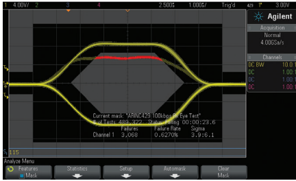
Figure 2: Eye-diagram mask test on an ARINC 429 serial bus using an Agilent 3000 X-Series oscilloscope.
