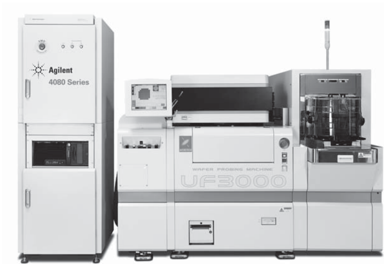
Figure 1.3. A production parametric tester is designed to optimize throughput
