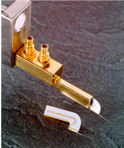
Figure 4.7. Ceramic bladed probe tips are the best solutions for on-wafer high-temperature measurement. Note: Photo courtesy of FormFactor
