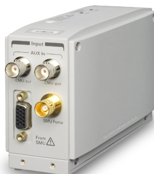
Figure 4.24. The inputs to the ASU, showing the two coaxial inputs (top), the triaxial input (from the force line of the MPSMU or HRSMU, lower right) and the control cable input (also coming from the MPSMU or HRSMU, lower left).
