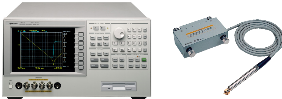
Figure 8.36. The 4294A or E4990A impedance analyzer and the 42941A impedance probe are both required to perform the advanced IV method of CV measurement.
