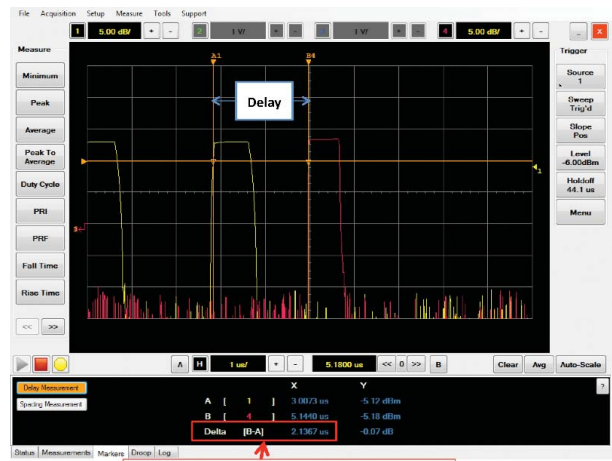
Delay measurement result
