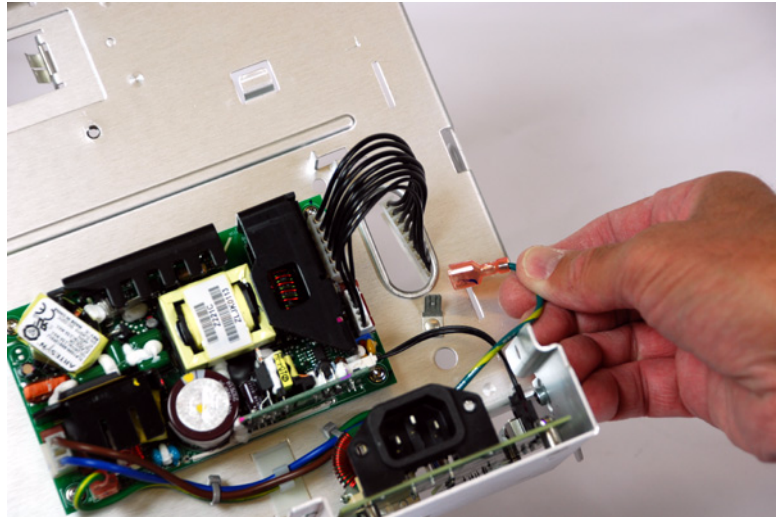
Figure 49 Disconnecting the ground wire
