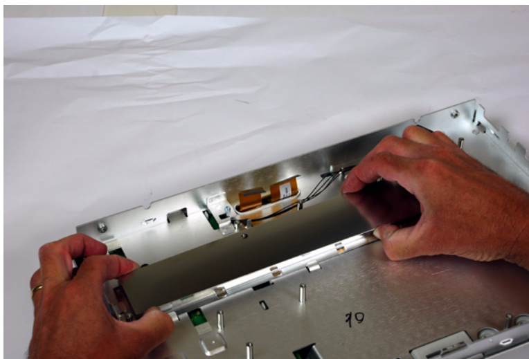
Figure 34 Removing the keyboard cable shield
