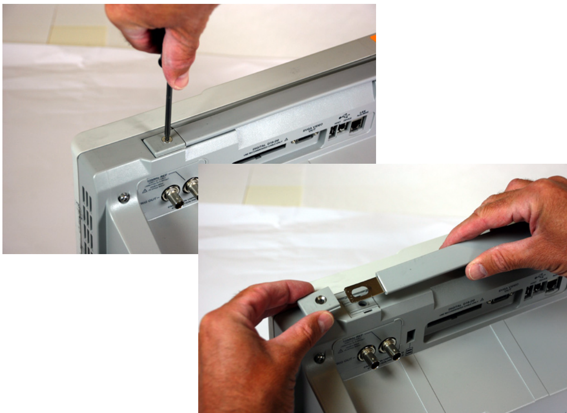
Figure 20 Removing the handle
