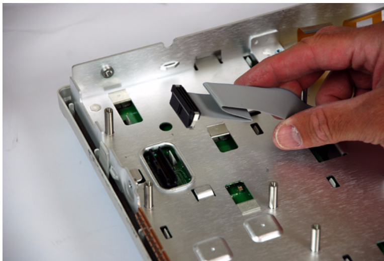
Figure 35 Disconnecting the keyboard cable
