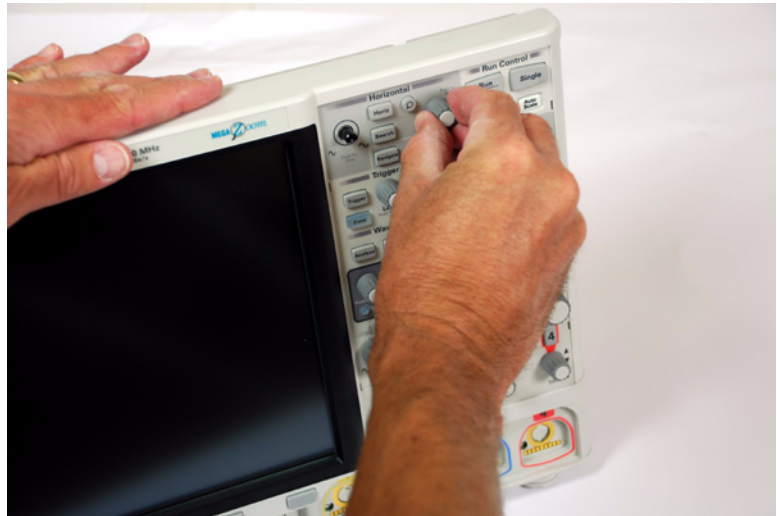
Figure 33 Removing the front panel knobs
