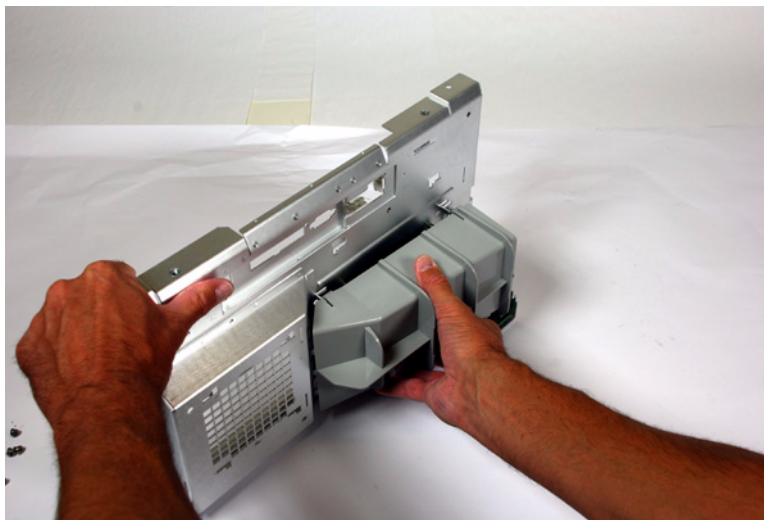
Figure 48 Removing the air duct
