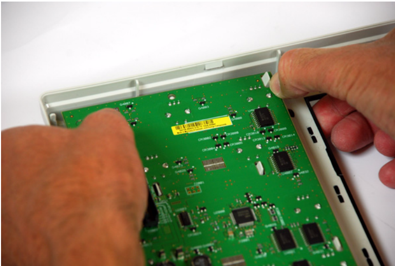
Figure 41 Removing the keyboard
