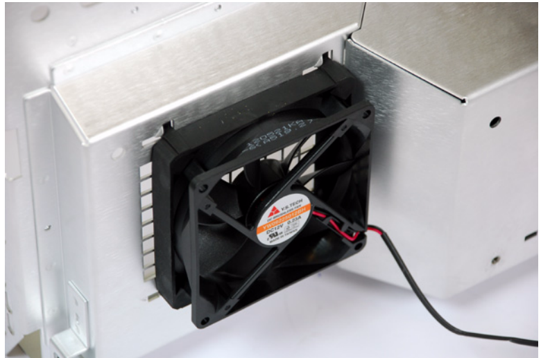
Figure 45 Removing fan assembly
