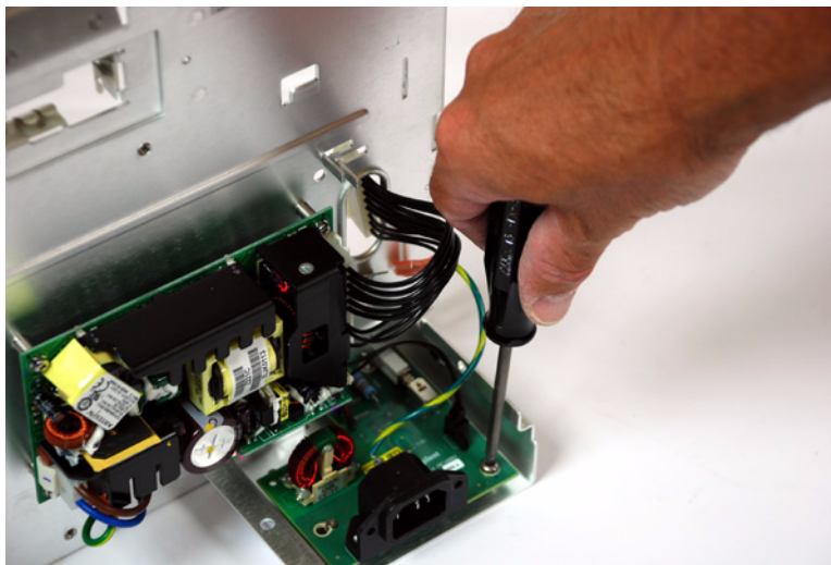
Figure 50 Removing the line filter board
