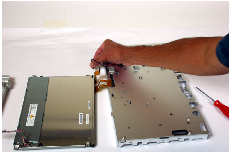
Figure 39 Disconnecting the backlight power cable
