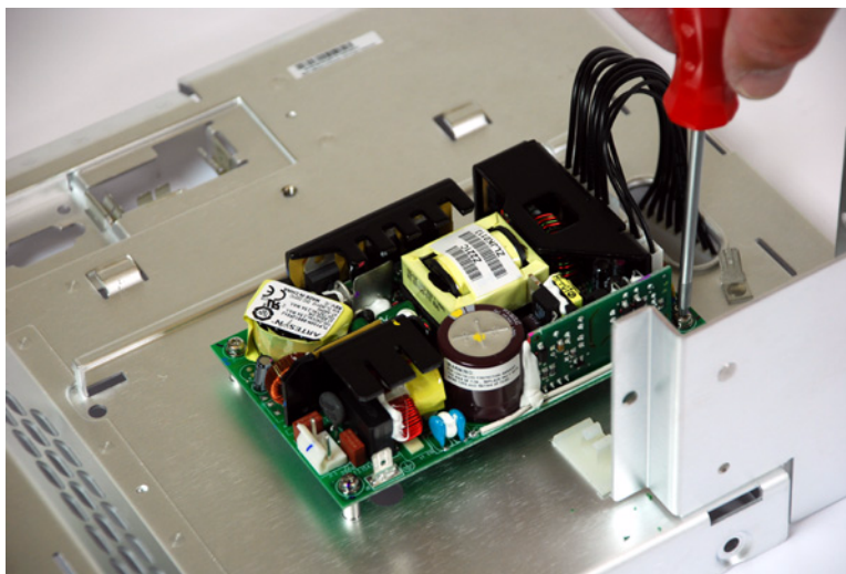
Figure 52 Removing the power supply
