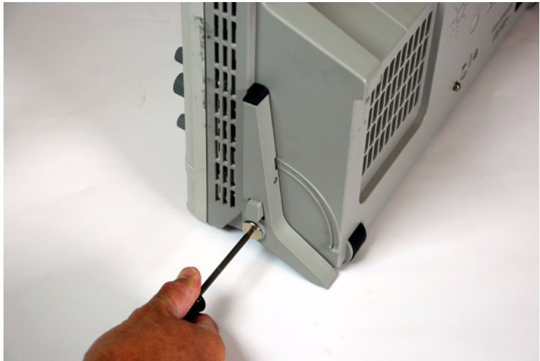
Figure 21 Removing adjustable legs
