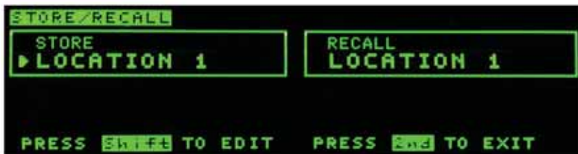
Figure 4. Selecting or recalling the store location can be done easily on the front panel of the 34450A.
