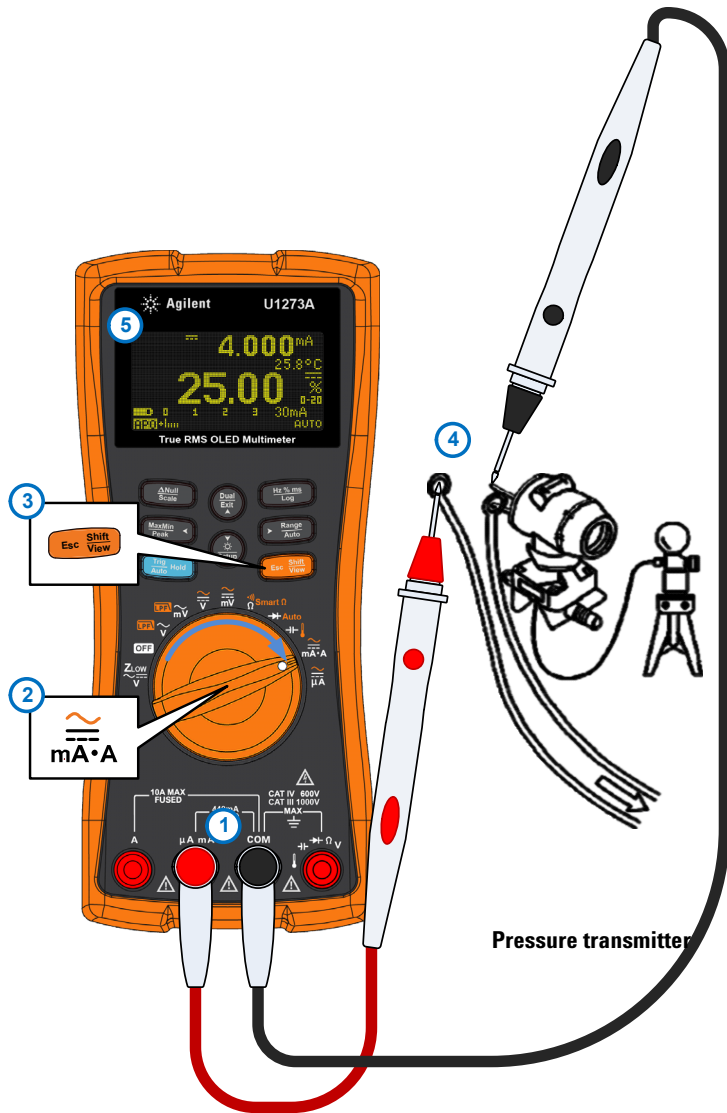
Figure 2-36 Measuring DC current using the 0-20 mA % scale
