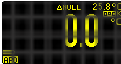
Figure 2-30 Temperature measurement without ambient compensation
