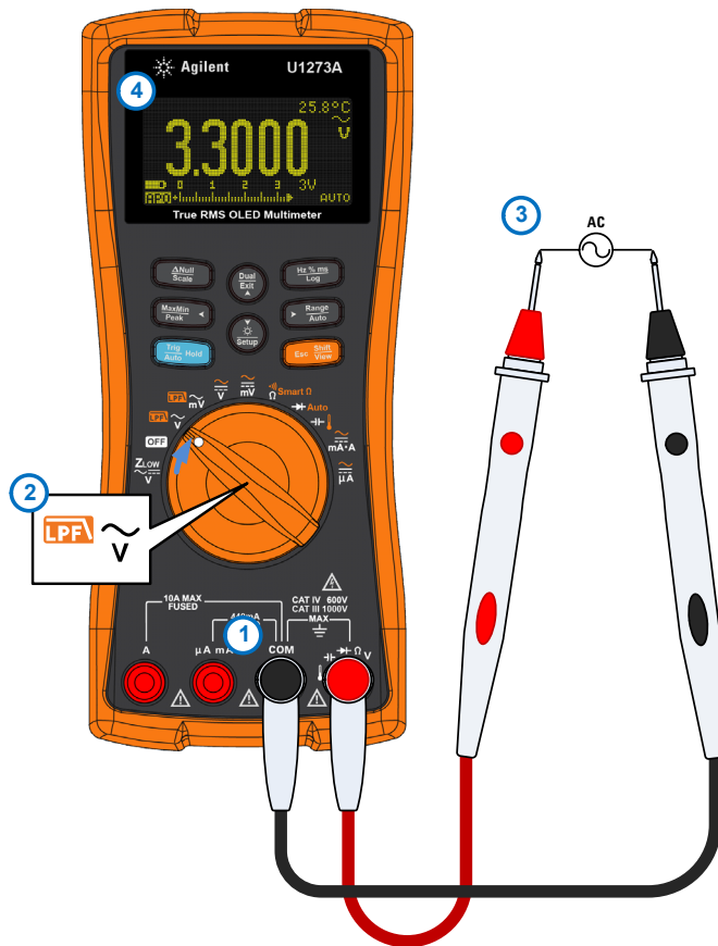
Figure 2-2 Measuring AC voltage
