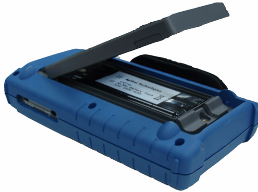
Figure 8-5 Remove battery pack cover without removing stand
