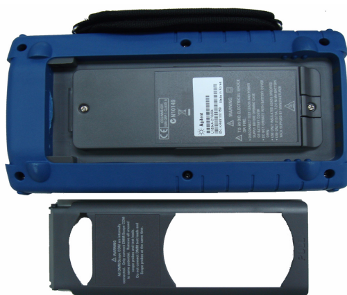
Figure 8-2 Disassemble the stand from the instrument
