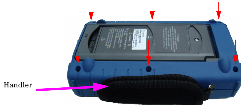
Figure 8-7 Remove screw from the rear cover
