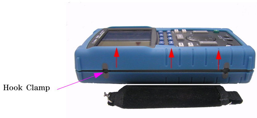
Figure 8-8 Remove handler from the instrument
