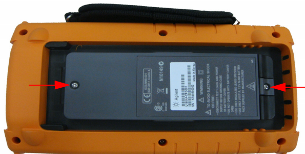
Figure 8-3 Remove battery cover screw
