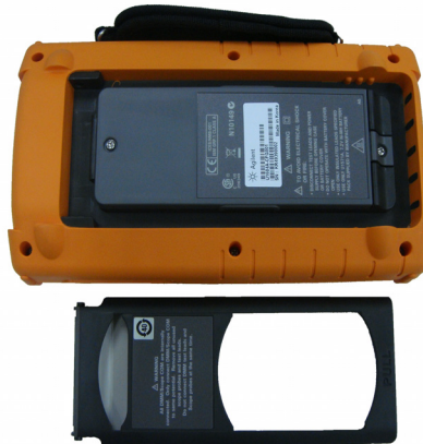
Figure 8-2 Disassemble the stand from the instrument
