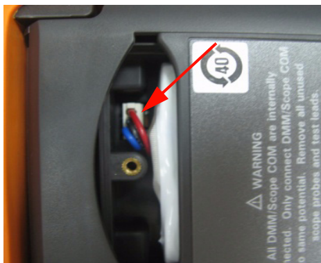
Figure 8-6 Unplug 2-wire connector with a tweezers.
