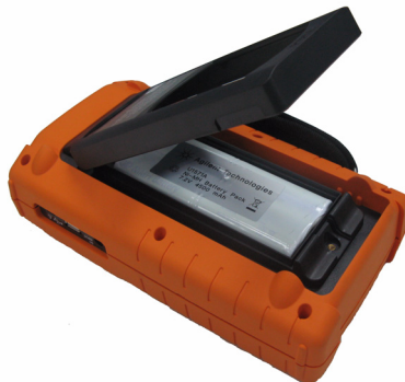
Figure 8-5 Remove battery pack cover without removing stand
