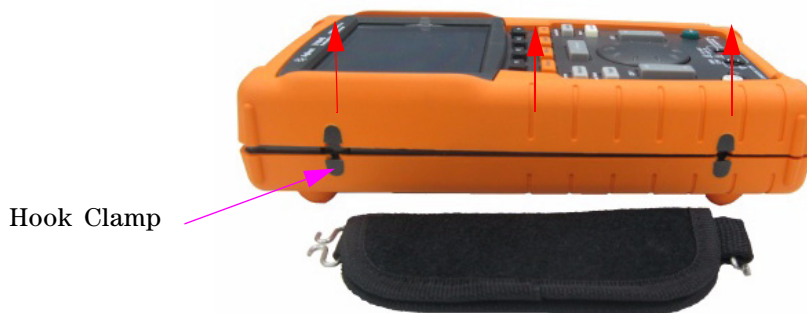
Figure 8-8 Remove handler from the instrument
