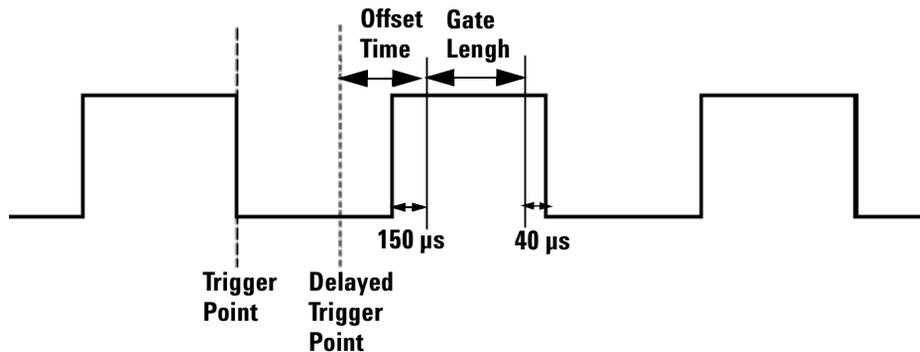
**Figure 2-2** Measurement gate
