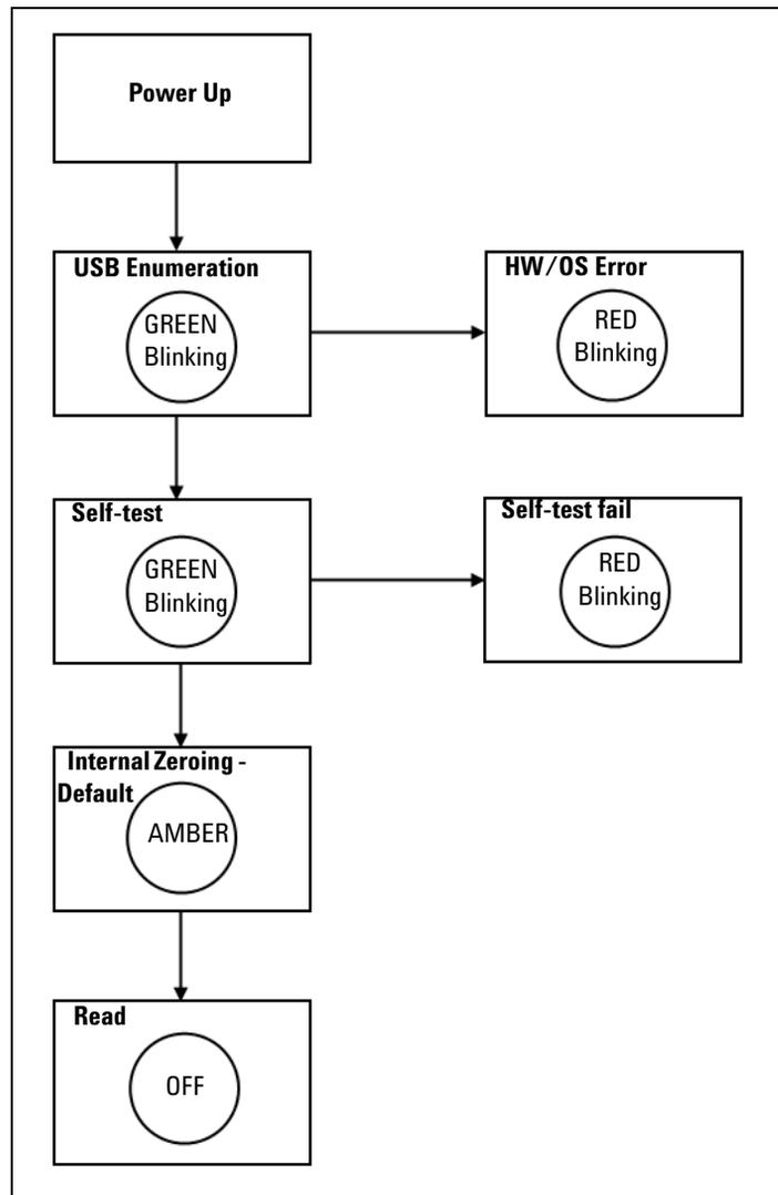
**Figure 1-1** LED indicator sequence during power-up
