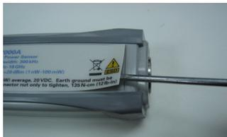
**2** Loosen three screws by using M2 to remove the housing.
