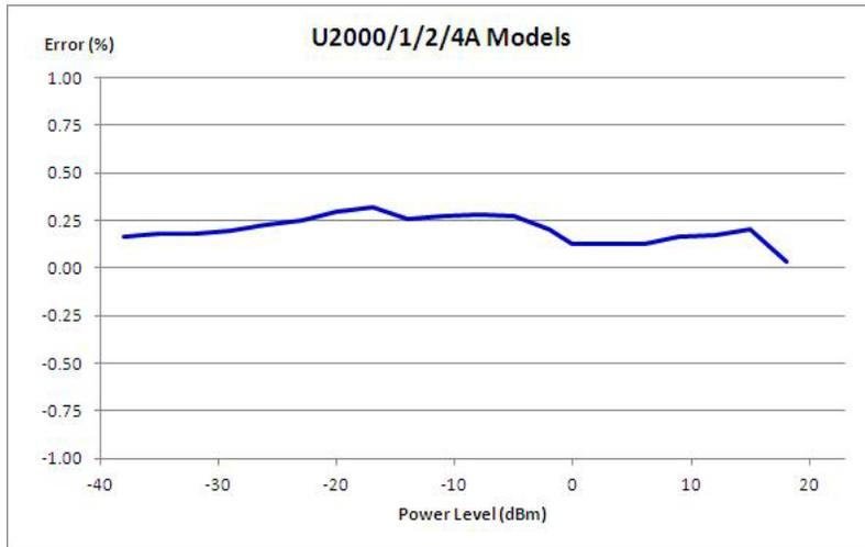
Figure 3-10 Typical power accuracy at 25 °C for U2000/1/2/4A models<sup>1,2</sup>
