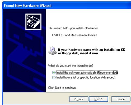
**Figure 1-5** Found New Hardware Wizard driver installation
