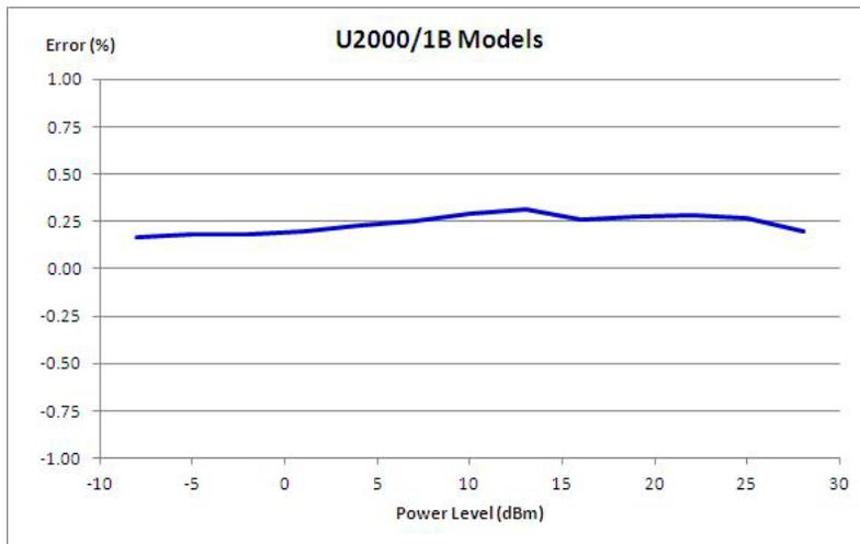
Figure 3-11 Typical power accuracy at 25 °C for U2000/1B models<sup>1,2</sup>
