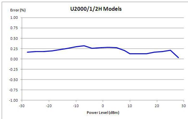
**Figure 3-12** Typical power accuracy at 25 °C for U2000/1/2H models<sup>1, 2</sup>
