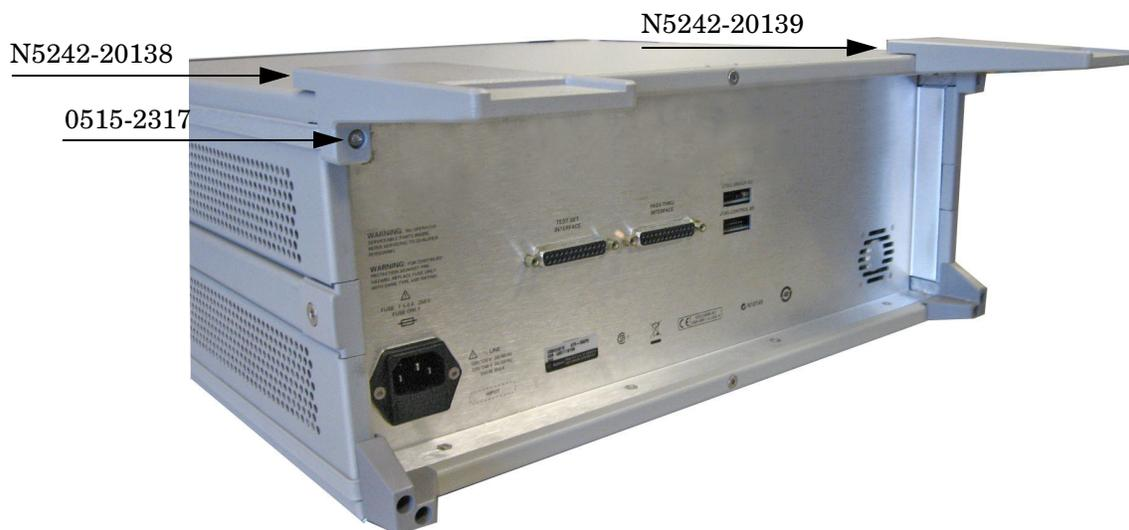
7. Place the PNA or PNA-X on top of the Test Set and ensure that the front frame of the analyzer is positioned slightly forward of the locks that are attached to the Test Set. Slide the analyzer back so the locks engage the front frame of the analyzer.
