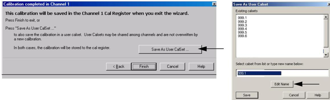
7. Repeat [step 1](#) thru [step 6](#) (1-Port Calibration Procedure) for Ports 2 thru 8. When finished, there should be 8 Cal Sets saved with the titles “999.1” thru “999.8” (8-Port).
