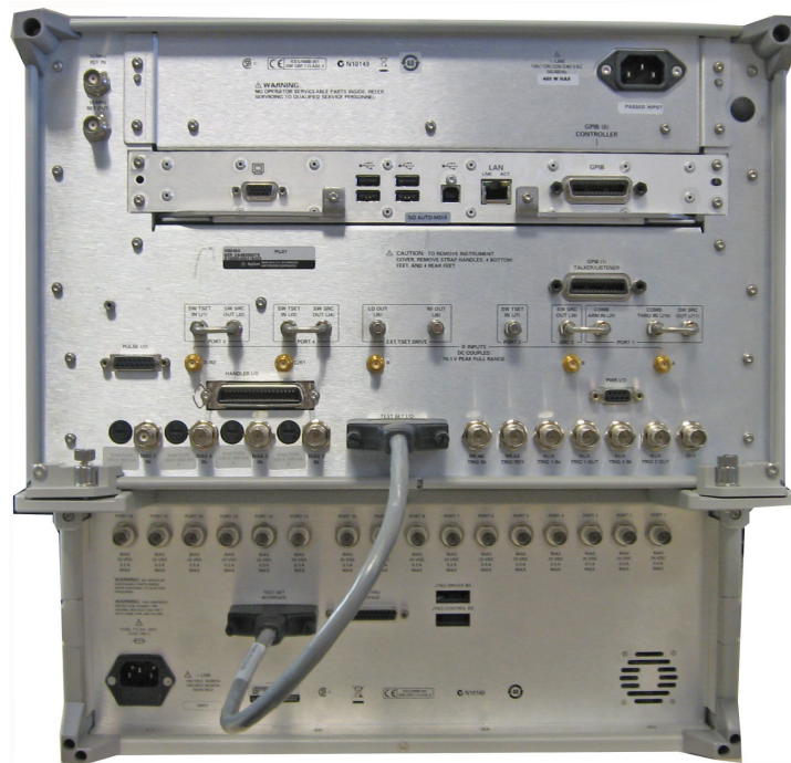
Figure 19 Test Set I/O Cable Connection
