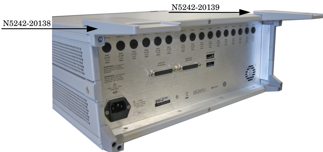
Figure 15 Install Locking Feet on Test Set
