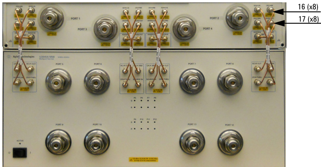
Figure 10 12-Port Interface Connections
