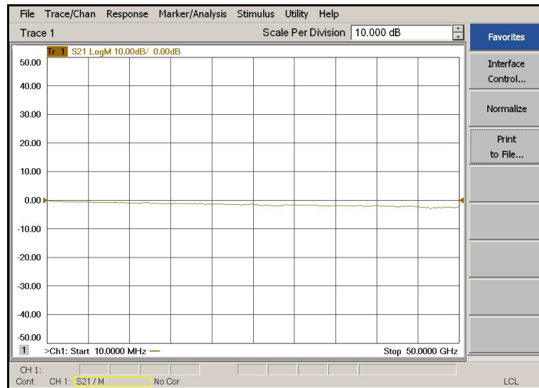
Figure 52 Source IN to CPLR THRU & RCVR OUT to CPLR ARM Path Response
