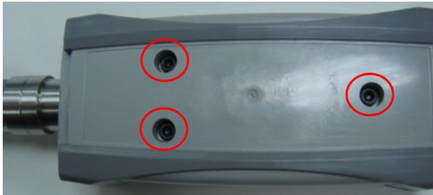
3 Replace the defective module with a new module.
