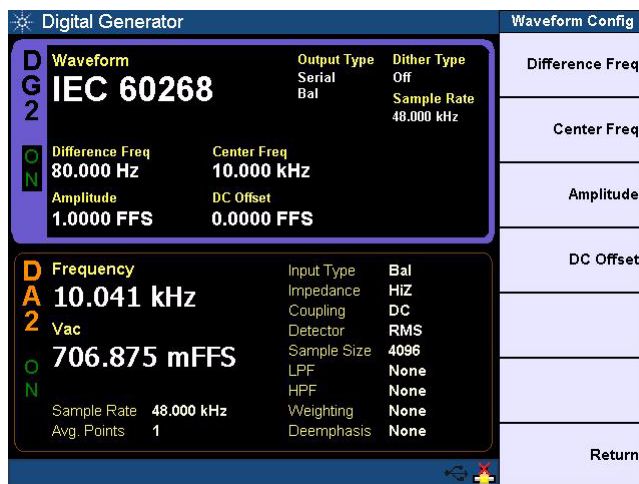
Figure 4-12 Digital generator DFD IEC 60268 waveform configuration
