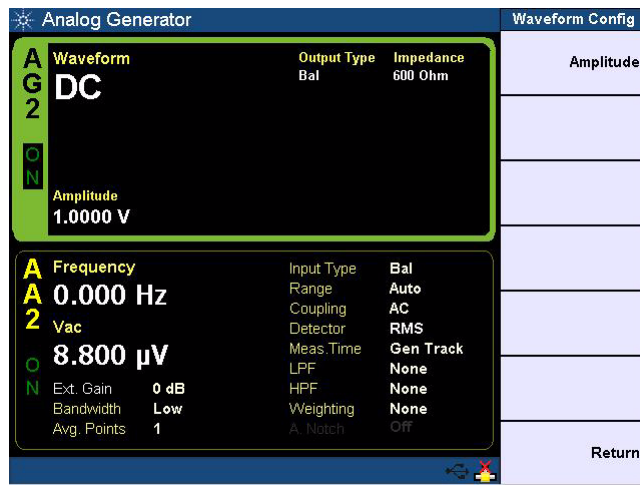
Figure 4-19 Analog generator DC signal configuration
