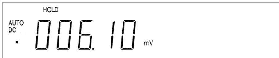
Figure 2-7 Typical refresh hold operation display
