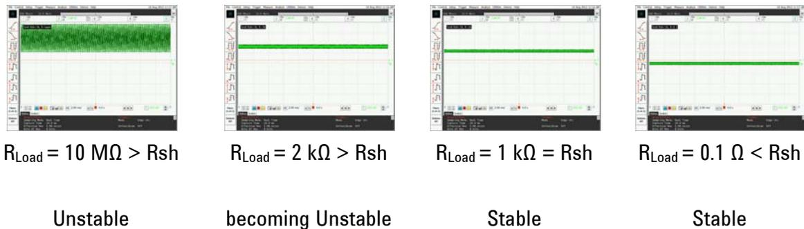
**Figure 9 I mode operation with various  $R_{Load}$**
