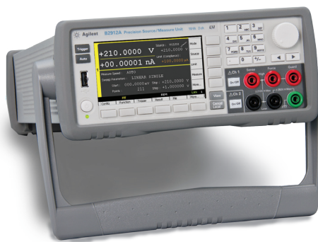
Figure 1. Image of the B2900A Series of SMUs and its circuit diagram to characterize a varistor
