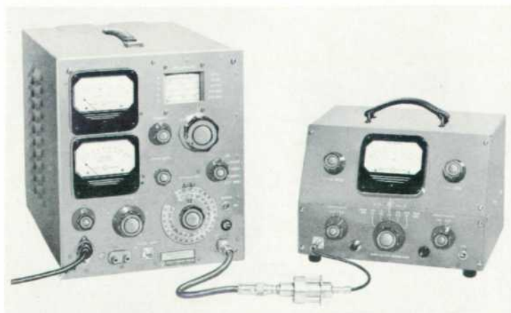
Figure 1. Set-up for standardizing signal generator output power using new -hp- Model 476A broad-band bolometer mount and new Model 430B power meter.
