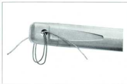
Fig. 6. Sensitivity of measurements can be increased by looping additional turns of measured conductor through probe. See details in text.
