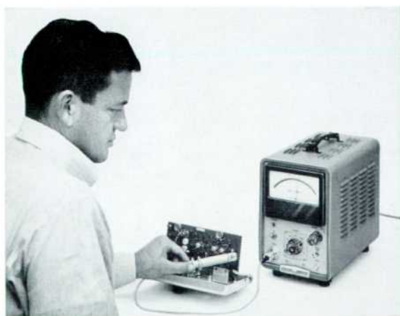
Fig. 1. New -hp- Model 428B Clip-on DC Milliammeter measures dc currents merely by clipping probe around current conductor. Instrument also has proportional output for alternating currents up to 400 cps, permitting a-c up to several amperes to be measured readily in heretofore difficult cases.
