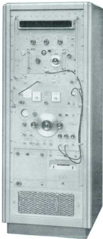
Fig. 4. Synchronizer-transfer oscillator-counter system packaged in cabinet. System measures frequencies with accuracy of parts in 10^8 . System shown is known as Dymec 5854 Frequency Measuring System.
