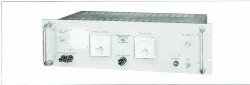
Fig. 1. Model DY-5796 Synchronizer produced by hp 's Dymec division enables frequency measurements to be made automatically from 200 mc to 12.4 gc with hp transfer oscillator and frequency counter. Unit is particularly valuable when measured frequency is drifting or has residual f-m .
