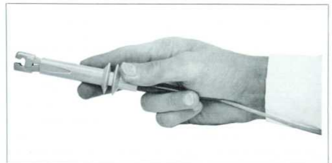
Fig. 4. Clip-On probe operates by flanges on probe body.
